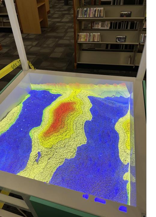
This piece uses Augmented Reality technology to explore how water moves through landscapes! A scanner sends information to a projector that shines down on a sandbox.
