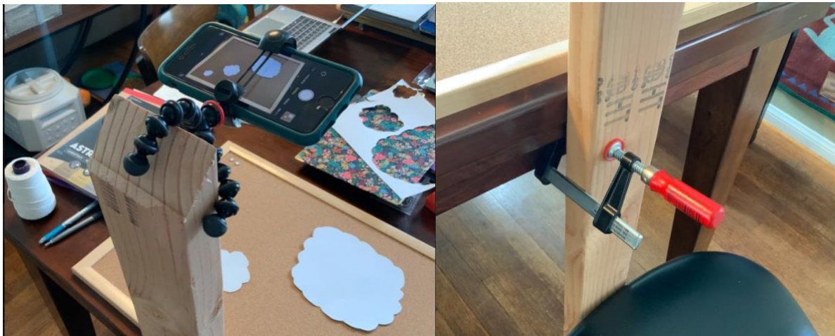
Figure 1: Left, flexi-tripod gripping wooden plank. Right, clamp holding plank to my table to get the phone camera at the right height.
